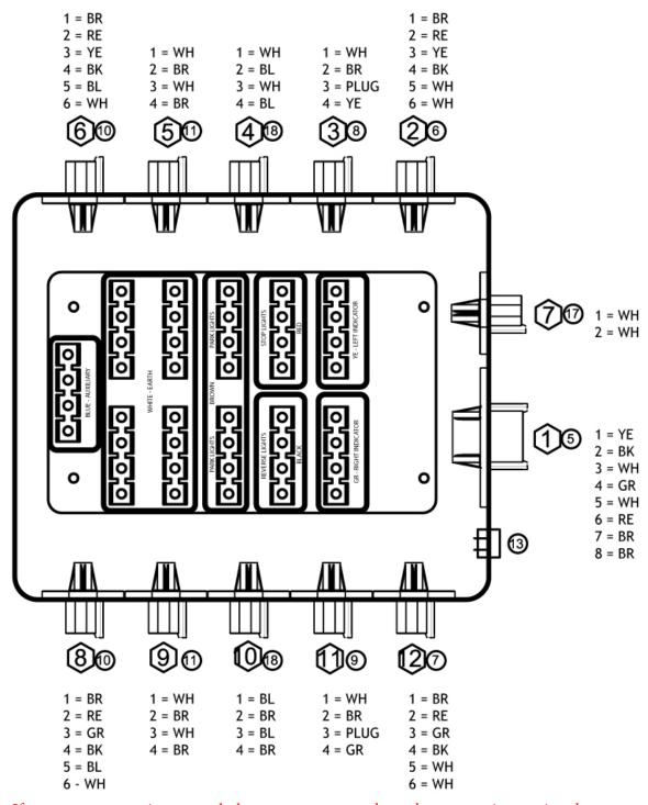
Note: If a connector port is not used please ensure to purchase the appropriate cavity plug for proper sealment from water and dust ingress.
