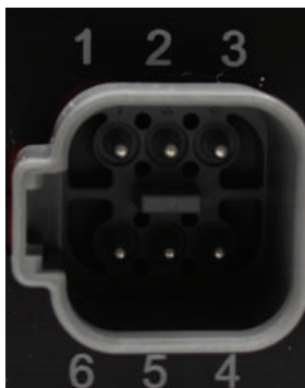
Connected using Industry accepted DT Deutsch Connector
